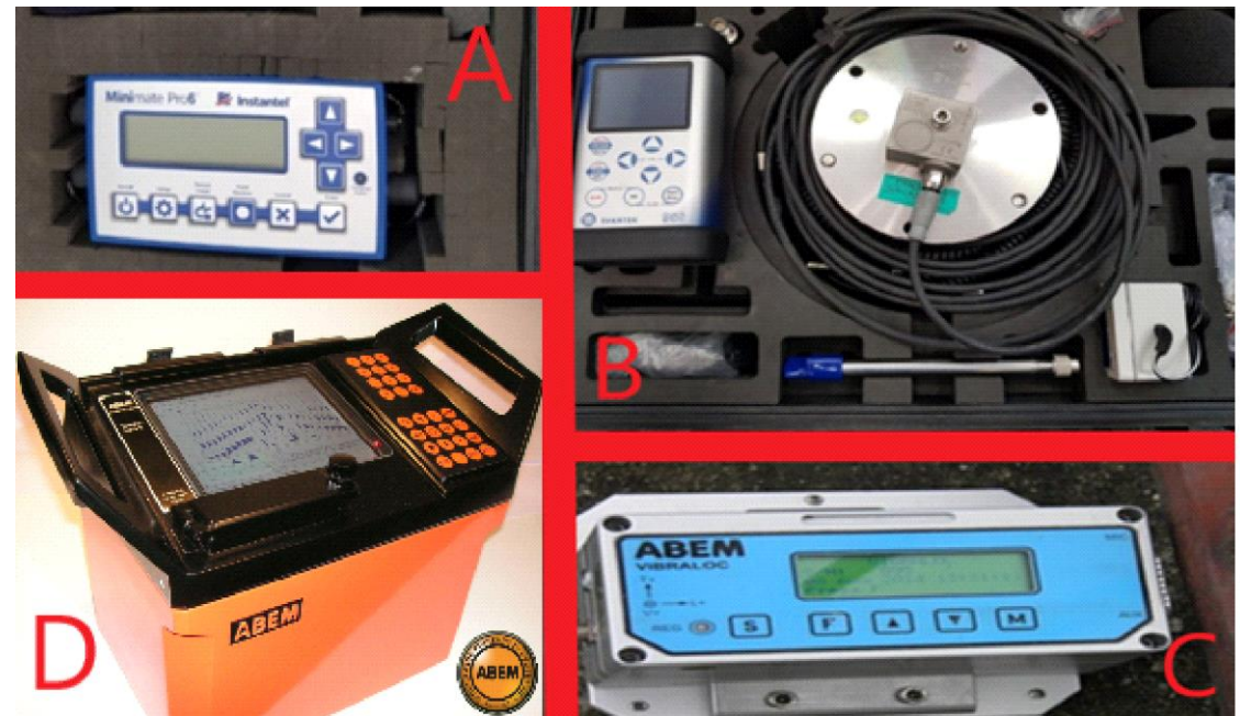
Fig. 4 Instruments used to measure technical seismicity and propagation seismic waves in rock massifs
