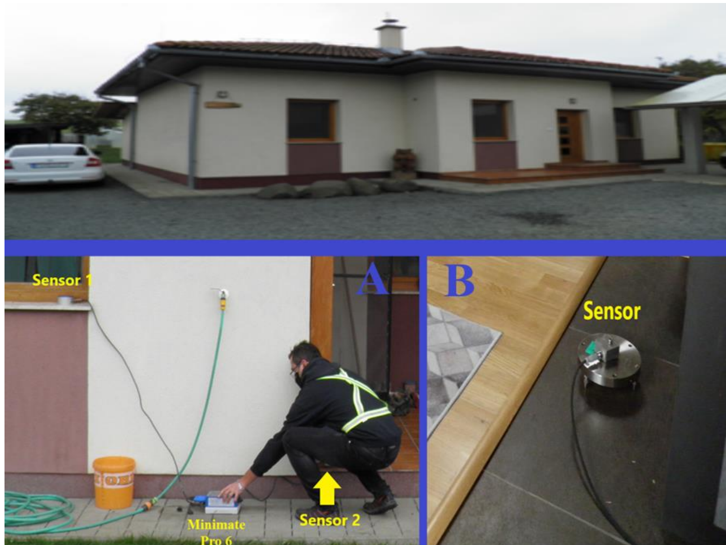
Fig. 7 Measuring station S2A - used Minimate Pro 6 measuring equipment to measure the effect of technical seismicity during CO 34 and CO 35 bench blasts on a residential building and S2B - used Svantek 958 measuring equipment to measure the effect of technical seismicity during CO 34 and CO 35 bench blasts on the residents of a residential building
