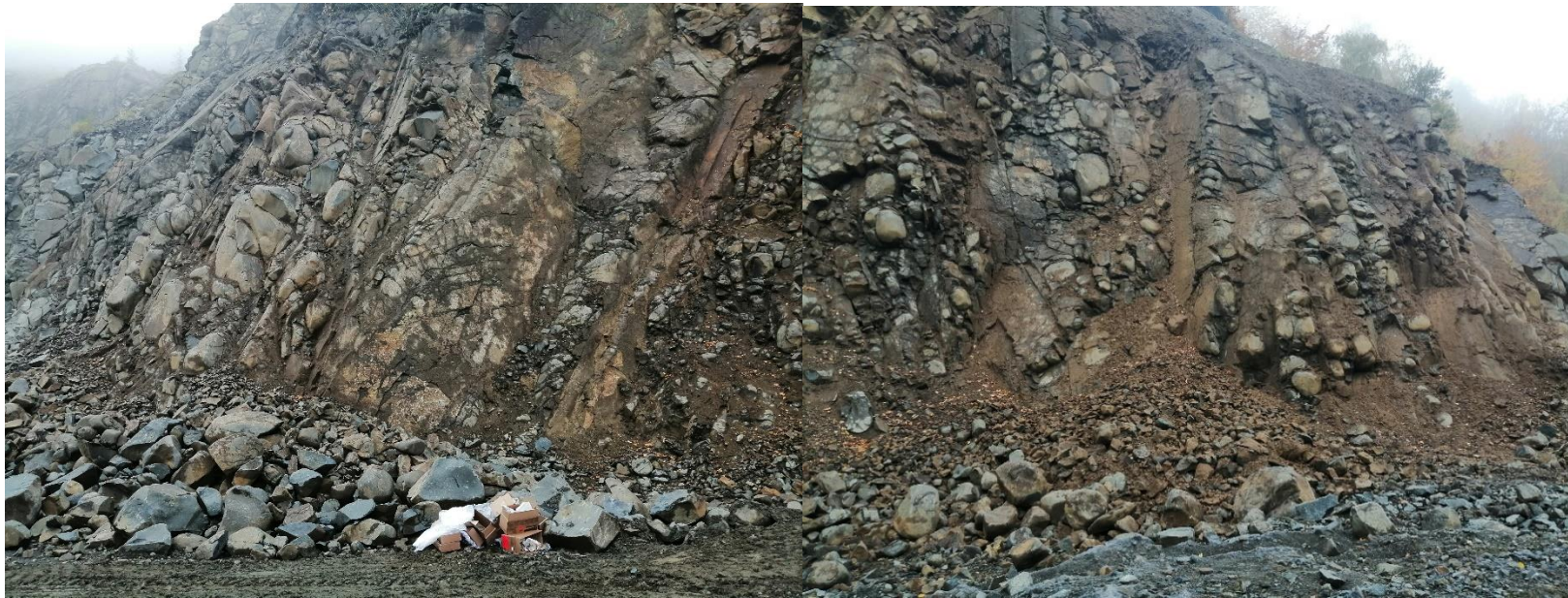
Fig. 3 View of the upper weathered part of the quarry Záhradné with spherical blocks of propylitized andesite
