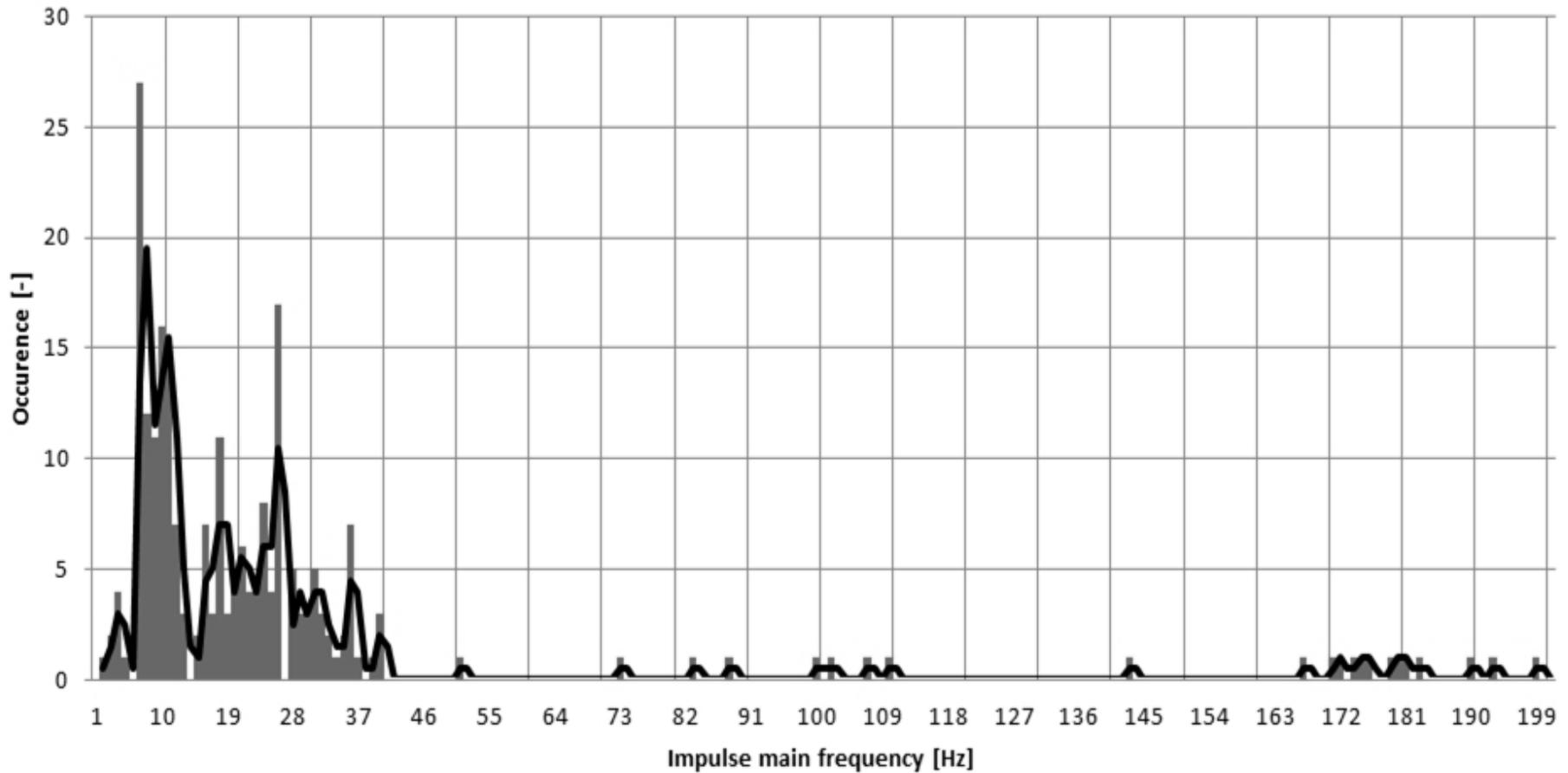
*Fig. 15 Statistical evaluation of the main frequencies of all the impulses from the successful fracturing tests (36 tested samples)*
