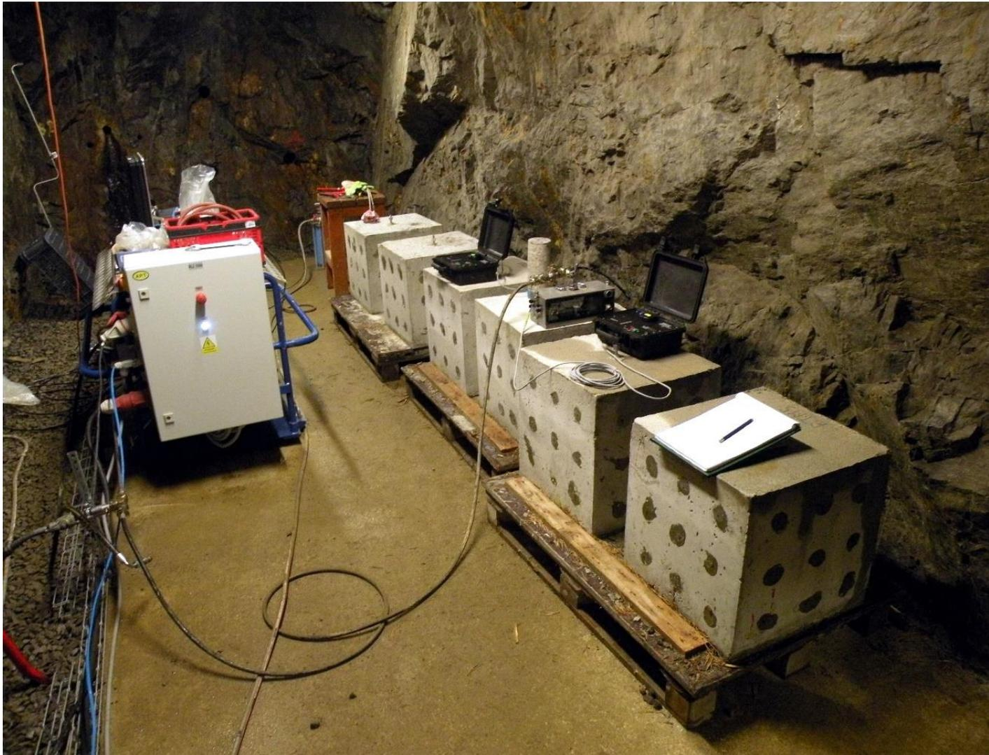
***Fig. 3 View into the testing chamber in underground laboratory Josef – several macro-samples prepared to be fractured by special hydraulic tool (standing to the left of the picture)***
