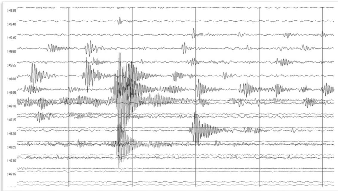
**Fig. 8** *Two-component recording of seismo-acoustic impulses during loading of the sample (x-axis time [s]; y - axis Amplitude of signal velocity vibration [mm/s])*
