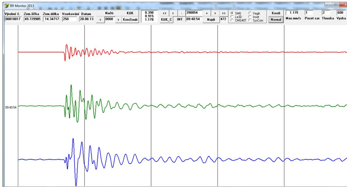
*Fig. 11 Detailed shape of the three-component wave recording of the course of the seismic response to deformation of the rock block during hydraulic fracturing ( x-axis time [s]; y - axis Amplitude of signal velocity vibration [mm/s])*
