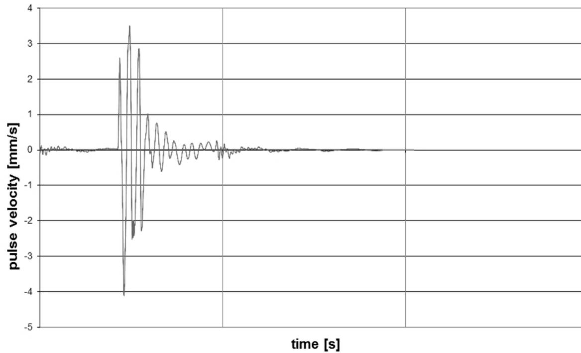
*Fig. 13 One-dimensional component of the recorded impulse on deformation of the rock block. The length of time interval is 3 s on the picture*
