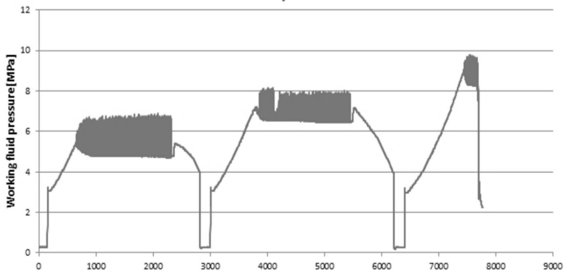
*Fig. 12 Typical working pressure curve of the fracturing liquid during the pulse test*
