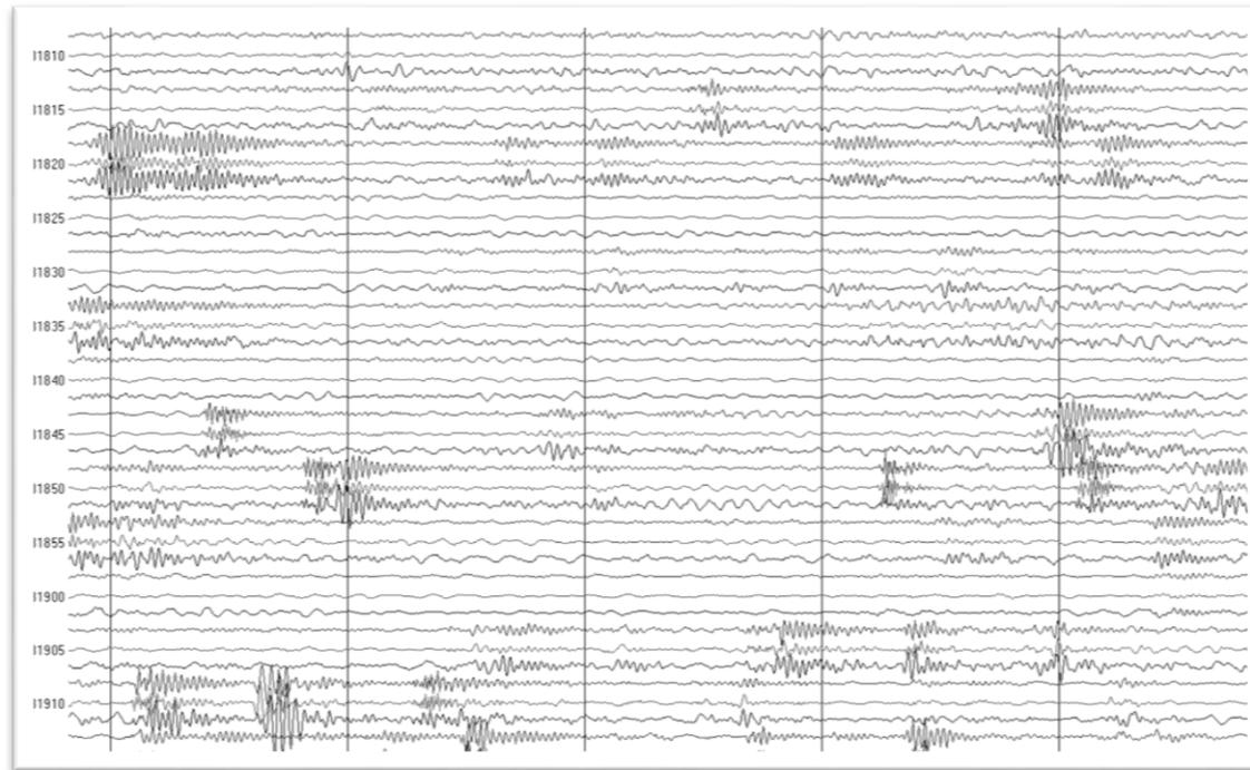
***Fig. 7 Regular time recording of seismic impulses in a normal daily regime at the site in-situ containing local seismic noise and impulse phenomena; one line corresponds to 5 s ( x-axis time [s]; y - axis Amplitude of signal velocity vibration [mm/s])***
