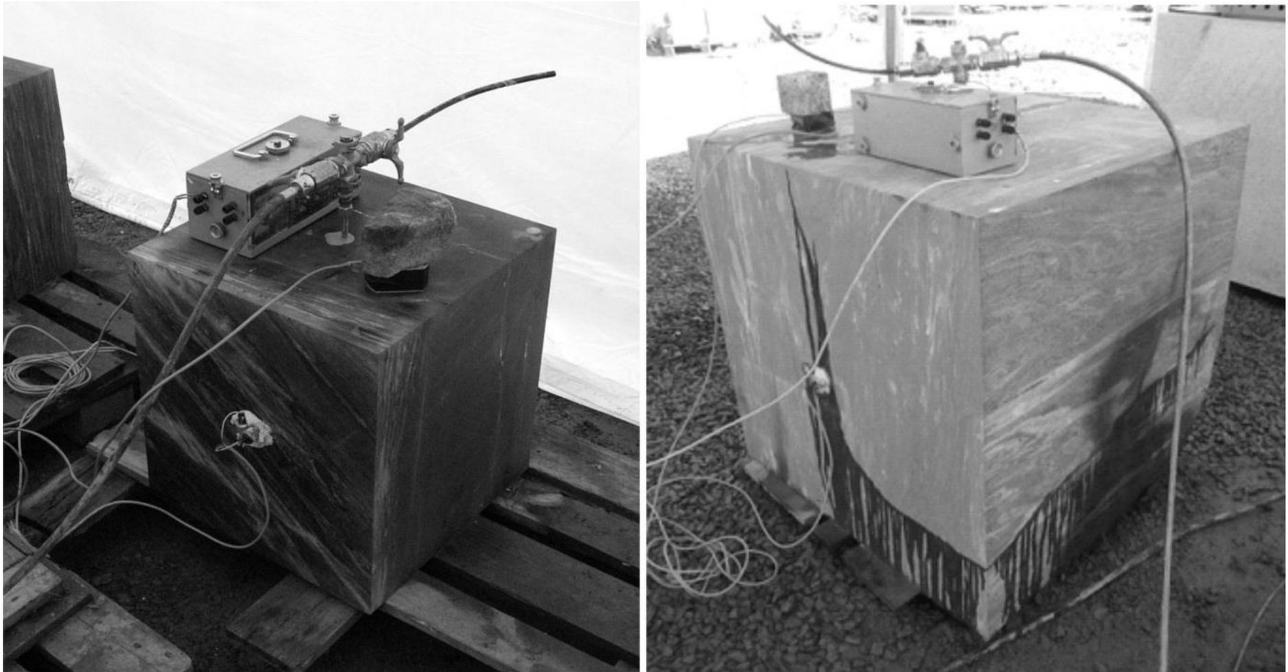
*Fig. 1 Example of instrumentation of the tested rock block by seismo-acoustic recorders, to the right is block after hydraulic test with visible pressure fluid outflow*
