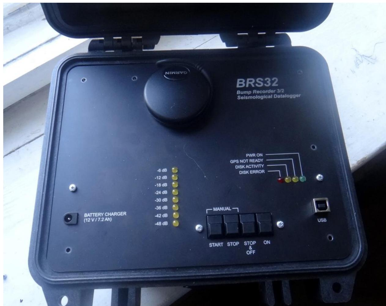
*Fig. 5 BRS32 recorder with internal battery and GPS receiver*
