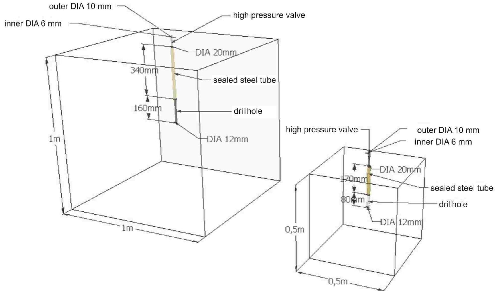
**Fig. 2 Scheme of inner instrumentation of the tested rock block application of hydraulic pressure**
