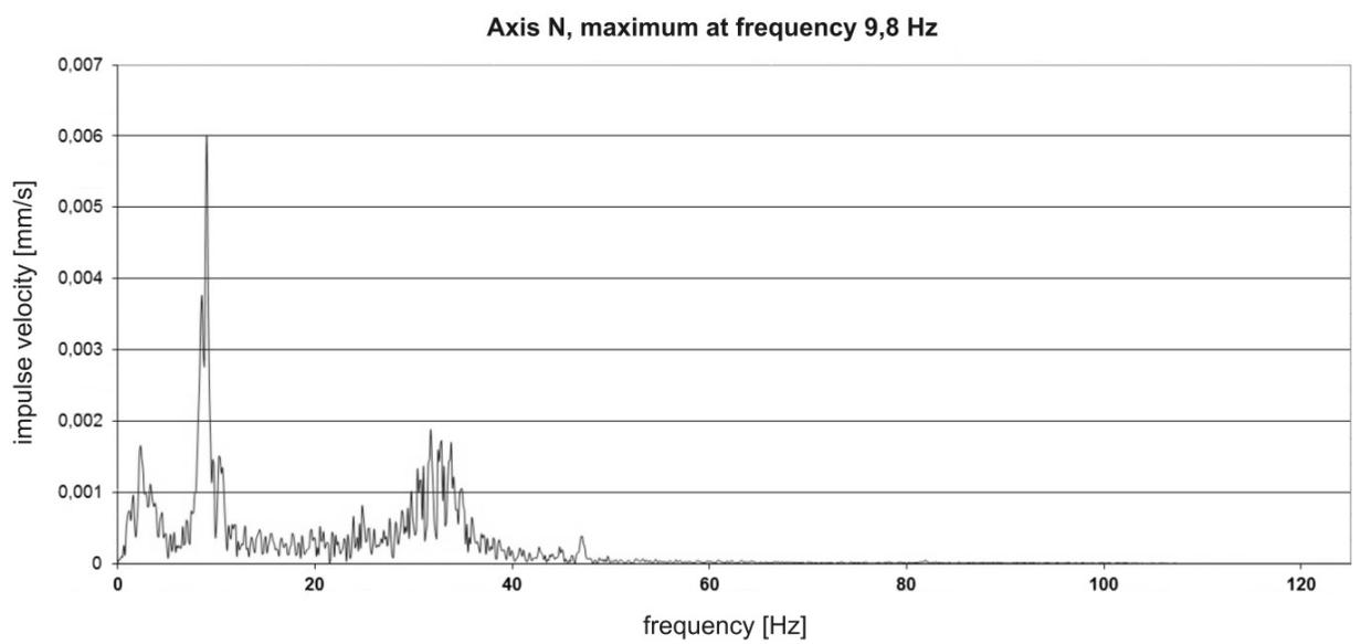
***Fig. 18 Frequency spectrum of the seismo-acoustic mixed recording – pulsator and deformation***
