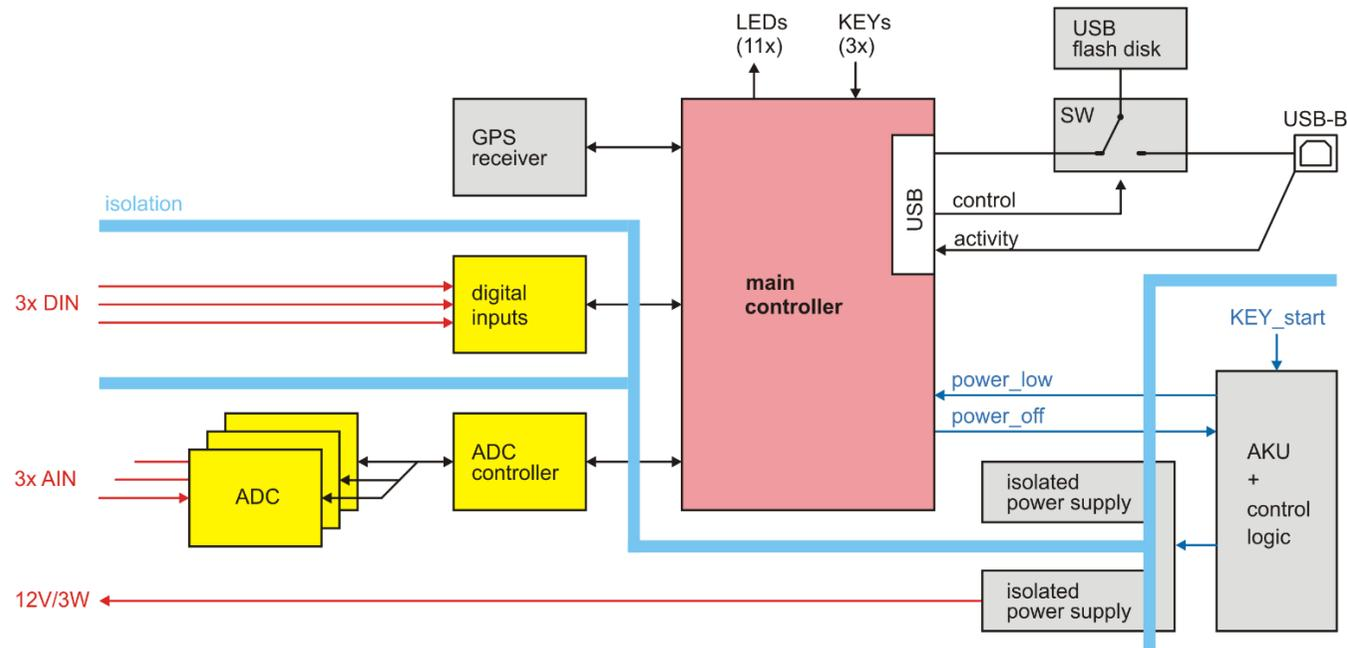
**Fig. 6 BRS32 recorder scheme with internal battery and GPS receiver configuration**
