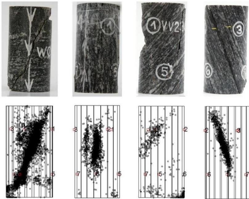
**Fig. 4** Location of the focal points of seismo-acoustic impulses in axial loading of a rock – borehole core. Size of cylindrical sample:  $r=50\text{mm}$ ,  $v=100\text{mm}$  (taken from Petružálek et al. 2008)
