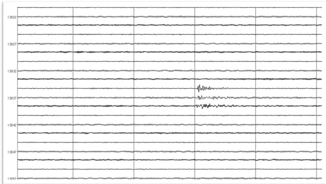
*Fig. 10 Recording of a seismic phenomenon on three components for which the distribution of the individual phases of the recorded seismic response to the impact is apparent ( x-axis time [s]; y - axis Amplitude of signal velocity vibration [mm/s])*
