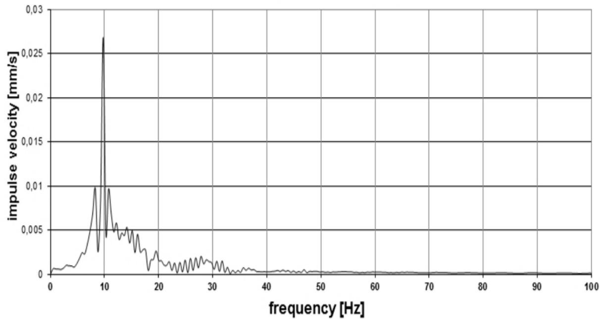
*Fig. 14 Frequency spectrum of the seismo-acoustic impulse on the formation of a new fracture*
