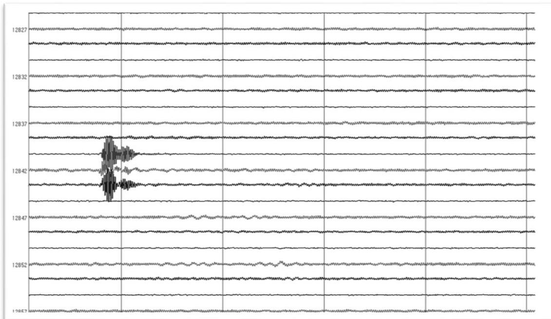
**Fig. 9** *Recording of the seismic response to a single deformation of the rock block in three components (x-axis time [s]; y - axis Amplitude of signal velocity vibration [mm/s])*
