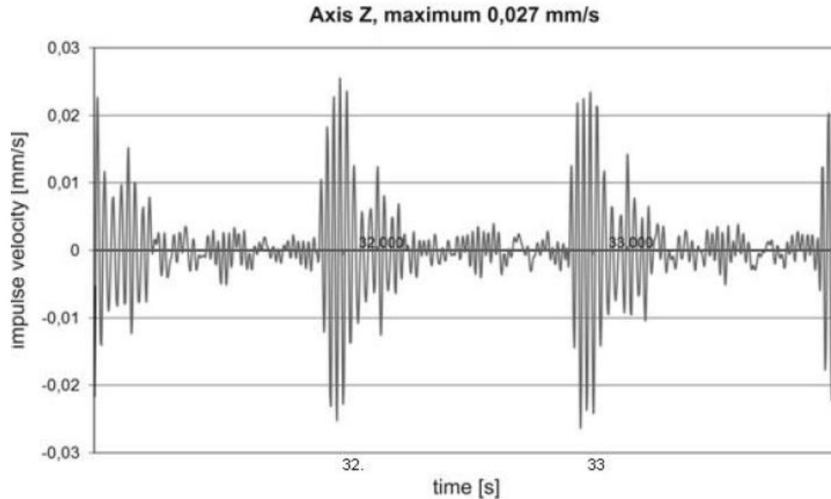
***Fig. 16 Seismo-acoustic recording of the effect of the pulsing equipment on the rock block***
