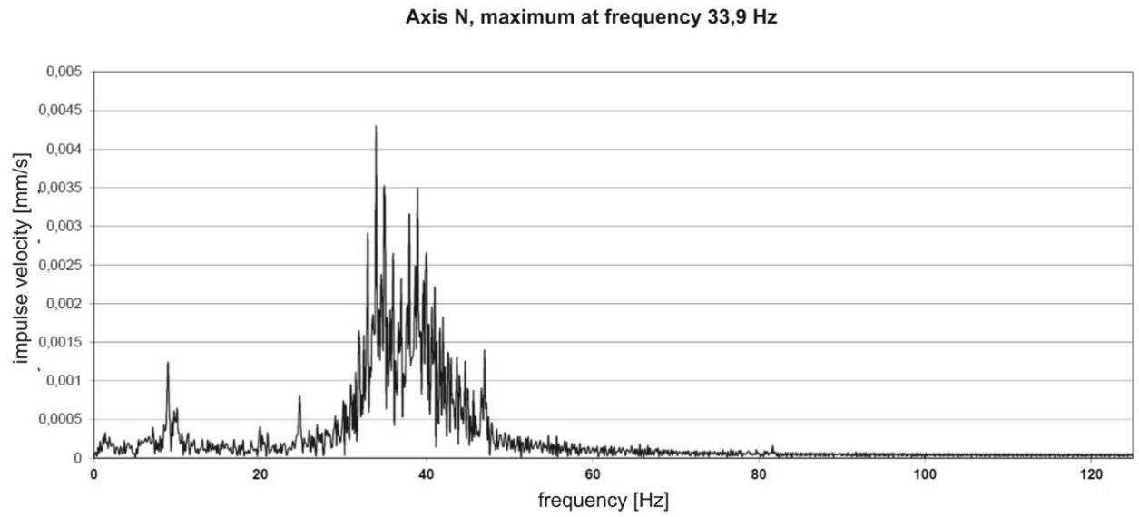
***Fig. 17 Frequency spectrum of the seismo-acoustic recording of the working pulsator***
