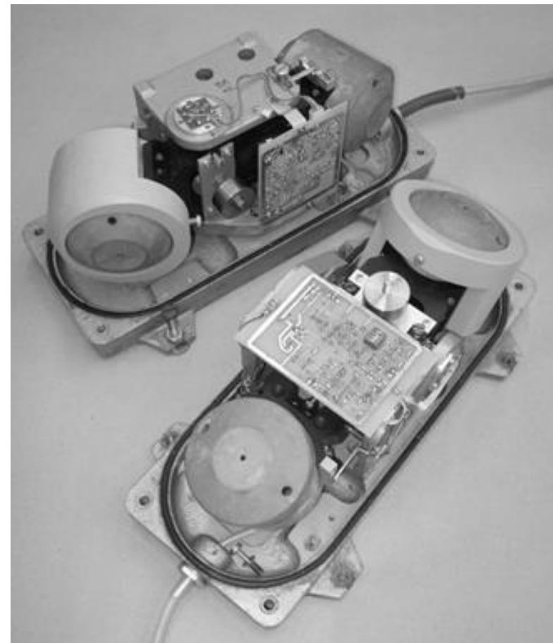
Fig. 1 The S-5-SR sensor recording rotational components of ground vibrations around the vertical axis (at the back) and around the horizontal axis (in the front); both sensors without cover (photo: Kaláb)
