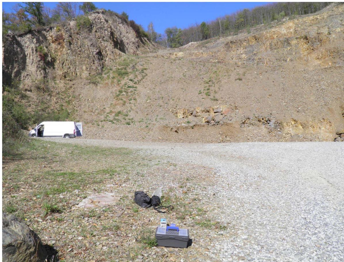
***Fig. 3 The second standpoint in Dargov quarry. Vibrograf ABEM Vibrac is located in 42 m distance from boreholes 1 a 2 at first and second blasts***
