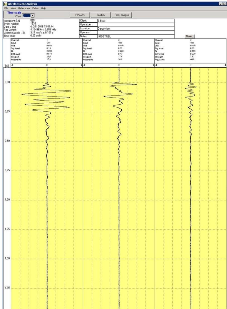
**Fig. 9** The record of particle velocities measured at the standpoint 2 - after the third blast. Channel 1 represents the z element, channel 2 represents the x element and y element is seen on the channel 3
