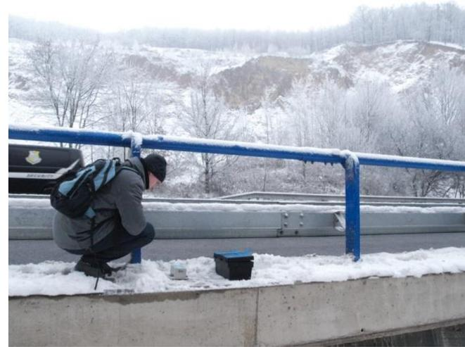
***Fig. 6 The third standpoint position on the supporting wall of road passing next to Dargov quarry. Vibrograf ABEM Vibraloc was located 126 m at third and fourth blast in the quarry Dargov***
