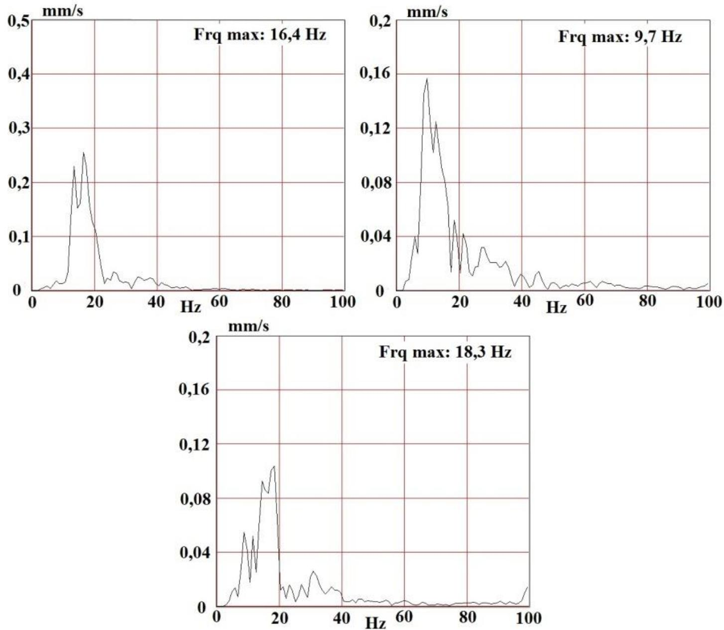
*Fig. 12 FFT analysis of the vibration record of wave in longitudinal, transverse and vertical direction measured at the standpoint 3 - after the third blast*
