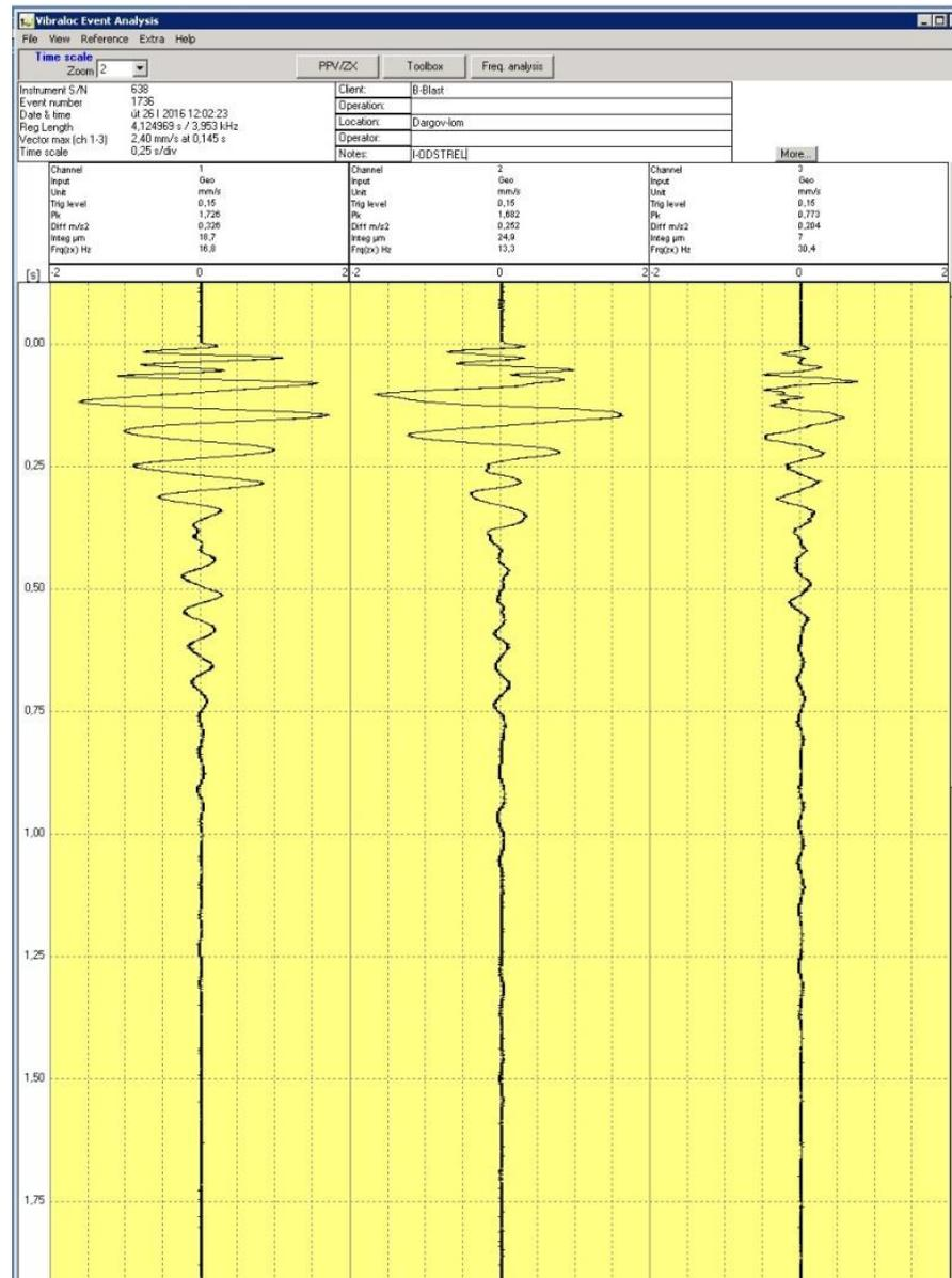
**Fig. 11** The record of particle velocities measured at the standpoint 3 - after the third blast. Channel 1 represents the z element, channel 2 represents the x element and y element is seen on the channel 3
