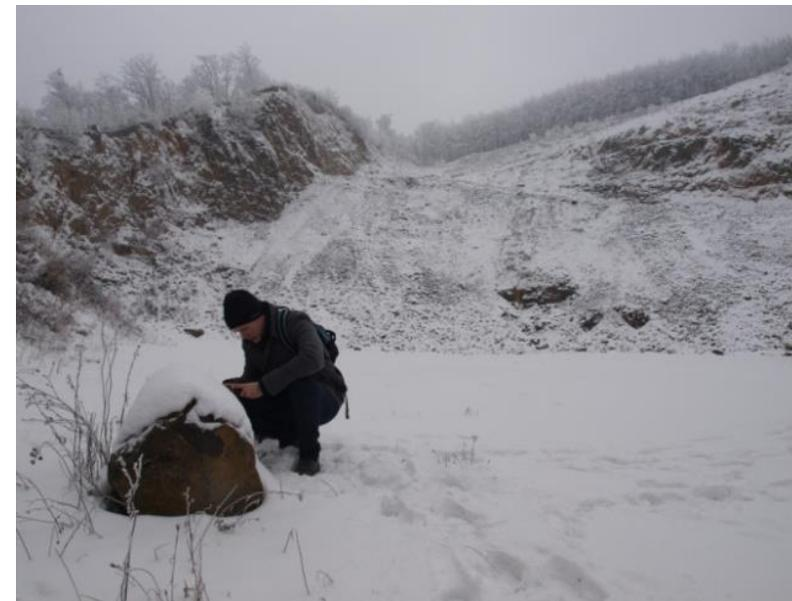
***Fig. 5 The second standpoint in Dargov quarry. Vibrograf ABEM Vibratloc is located in 90 m distance from boreholes 1 a 2 at third and fourth blasts***
