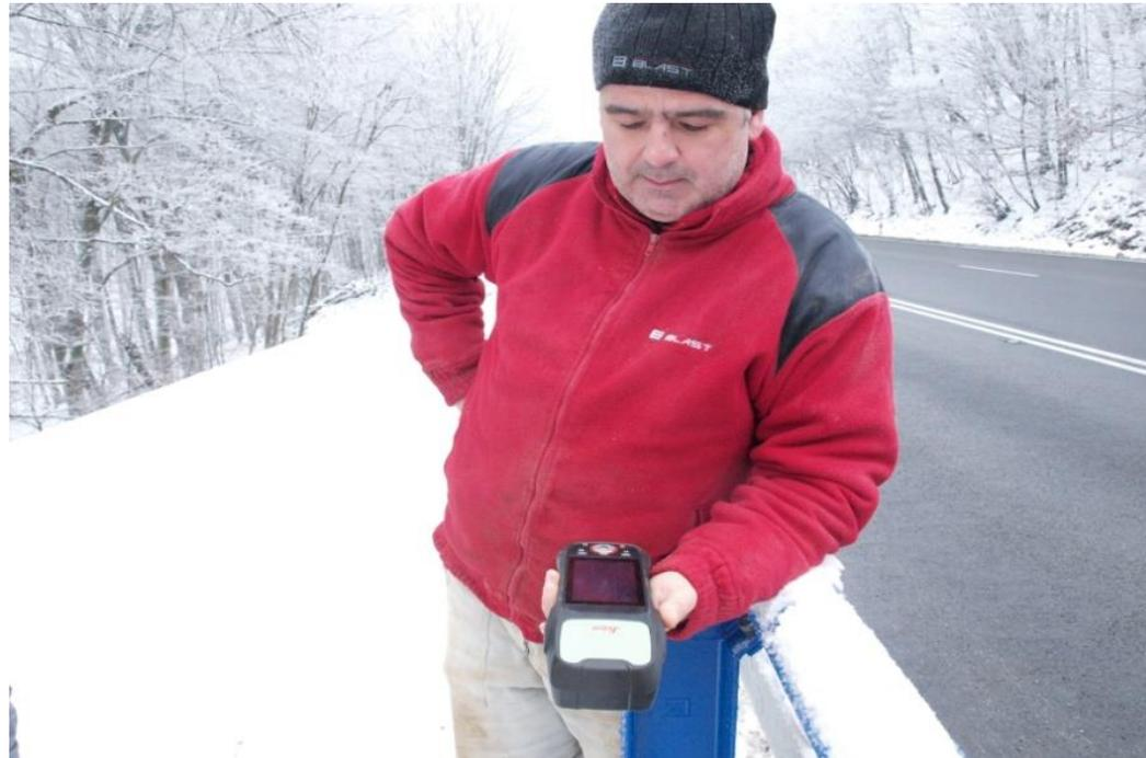
***Fig. 7 Localization of individual standpoints by Leica Zeno 20 device***
