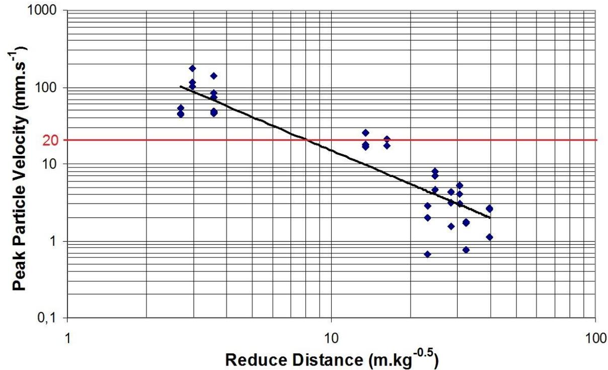
***Fig. 13 Derived trend of maximum components of particle velocity at reduced distance during test blasts in Dargov quarry – attenuation law of seismic waves. Blue dots show the maximum particle velocity measured during experimental blasts at standpoints 1, 2 and 3***
