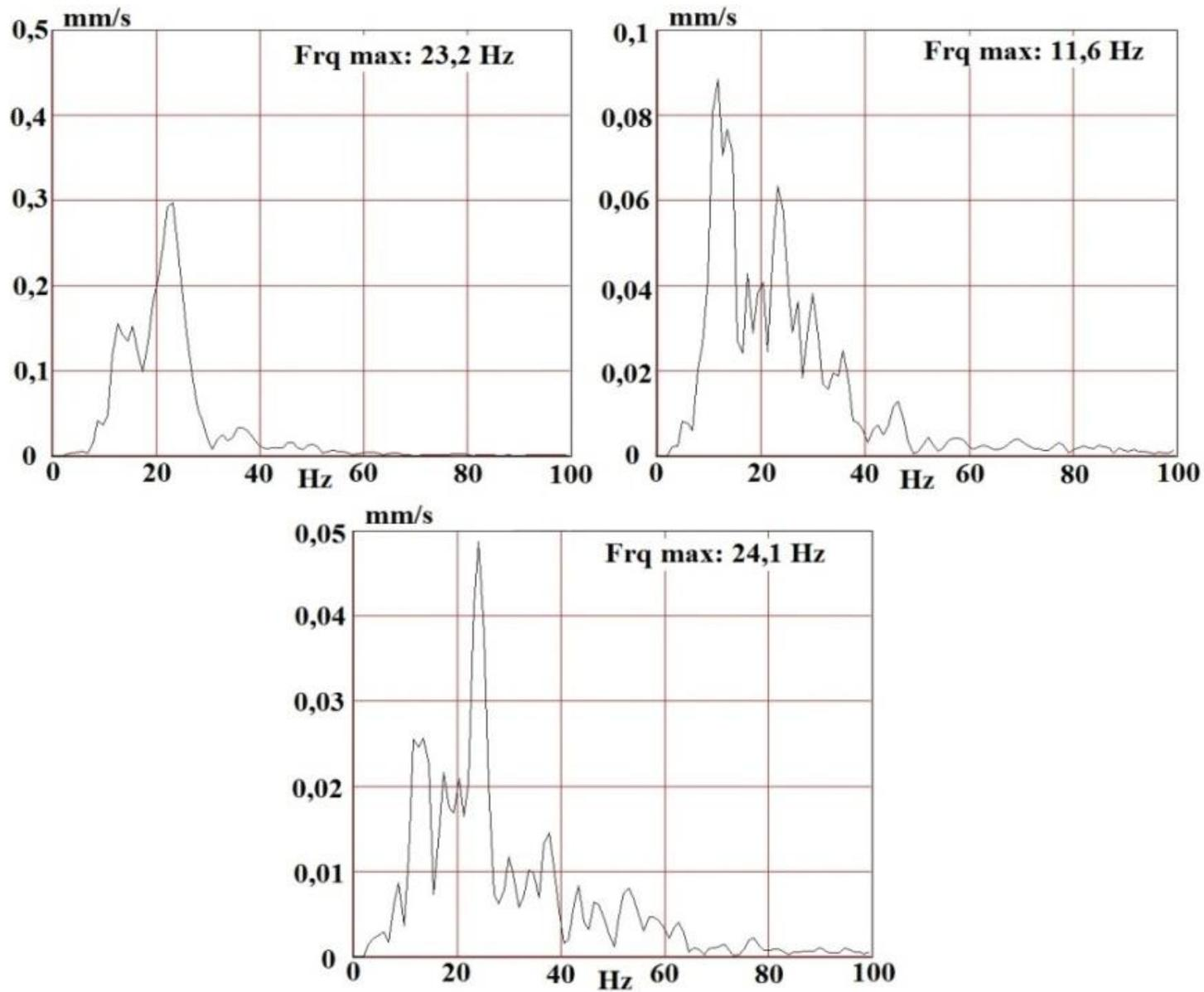
*Fig. 10 FFT analysis of the vibration record of wave in longitudinal, transverse and vertical direction measured at the standpoint 2 - after the third blast*
