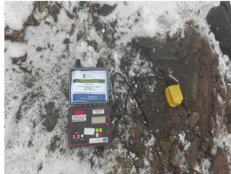
***Fig. 4 The first standpoint in Dargov quarry at third and fourth blasts. Vibrograf VMS 2000 is located 5.2 m from boreholes 1 a 2***
