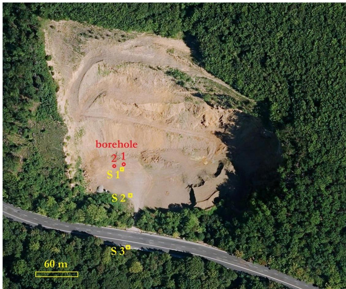
*Fig. 2 The location of boreholes 1 and 2 in relation to the standpoints 1, 2 and 3, where the first and second blasts were realized*
