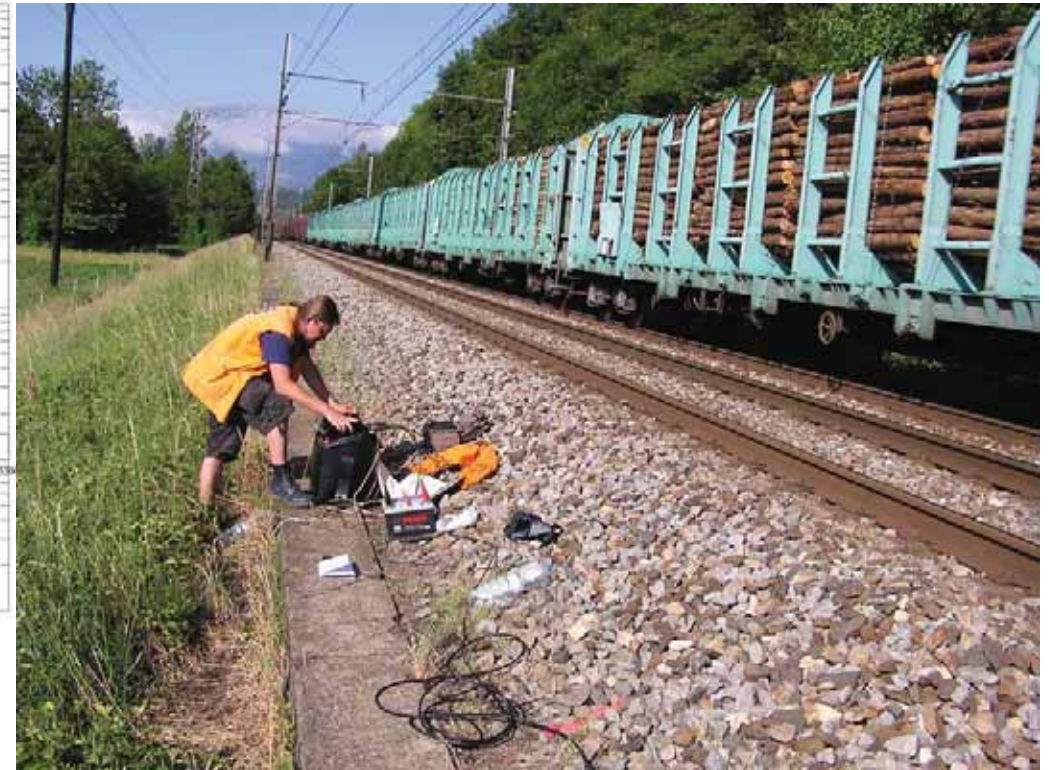
Fig. 6: The measurement using the seismic apparatus Terraloc. Montmélian, France.
