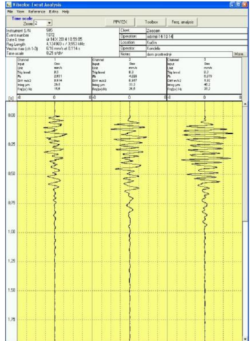
**Fig. 9a** The resulting record the particle velocity
