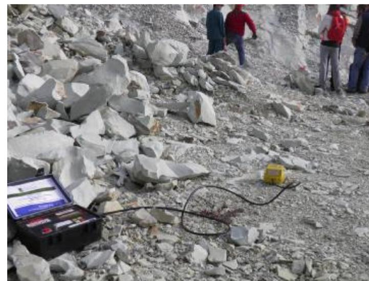
Fig. 2 Measuring opinion Kučín quarry – a position located, three-component seismometers GEOSPACE were placed 10.2 meters from the blast
