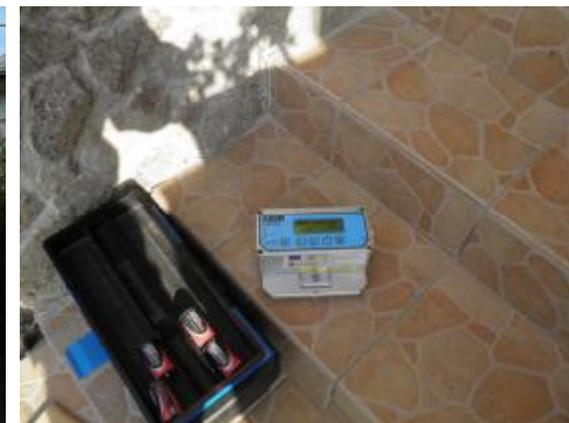
*Fig. 4b Seismometer was placed on a foundation wall in front of the house*
