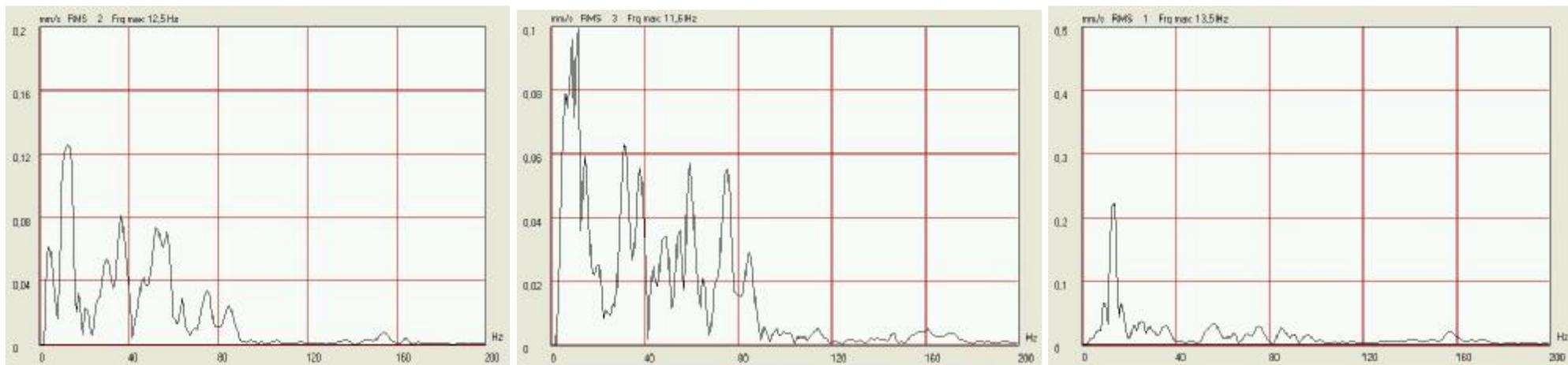
**Fig. 11 Frequency analysis of the vibration record of the individual components (in the longitudinal, transverse and vertical directions) measured on the measuring position 2 – residential building, on the 4. blast**
