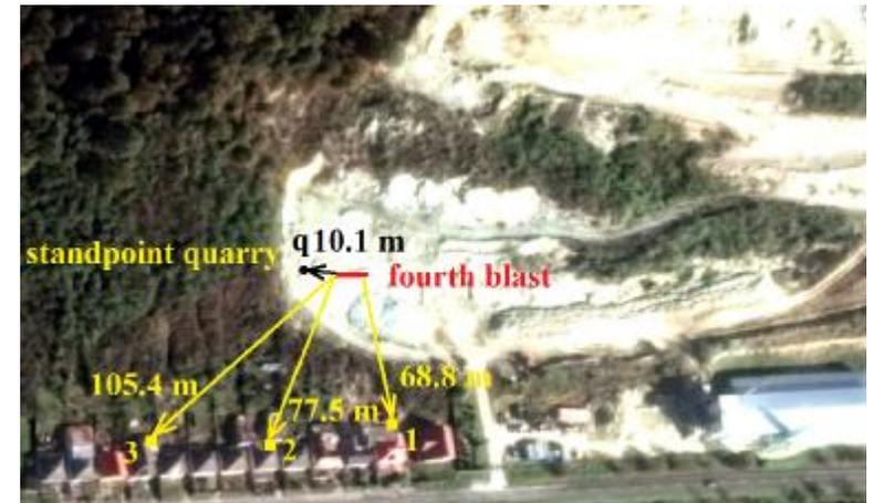
*Fig. 6 Position and distance fourth blast in the Kučín quarry in relation to the measuring standpoints in the Kučín village*
