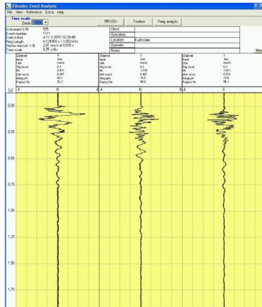
*Fig. 10 The resulting record the particle velocity of the components (in the longitudinal, transverse and vertical directions) on the measuring position 1 – residential house, on the 4. blast. The measured values are given in Table 3*
