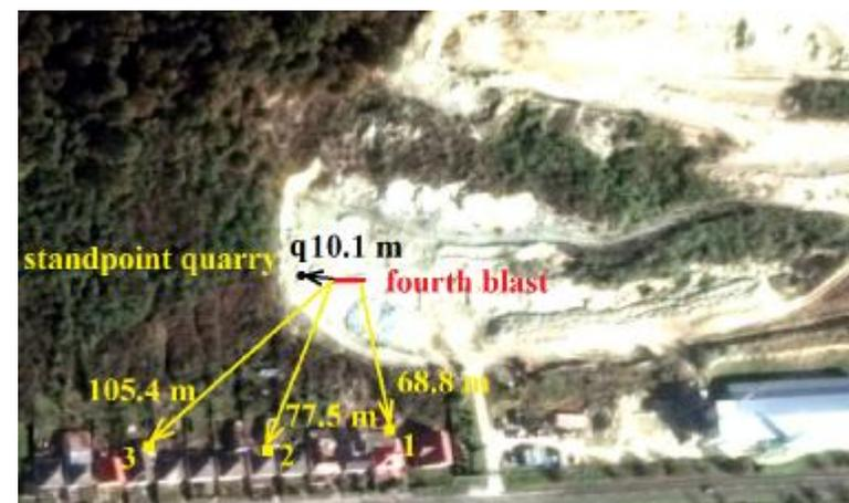
*Fig. 6 Position and distance fourth blast in the Kučín quarry in relation to the measuring standpoints in the Kučín village*
