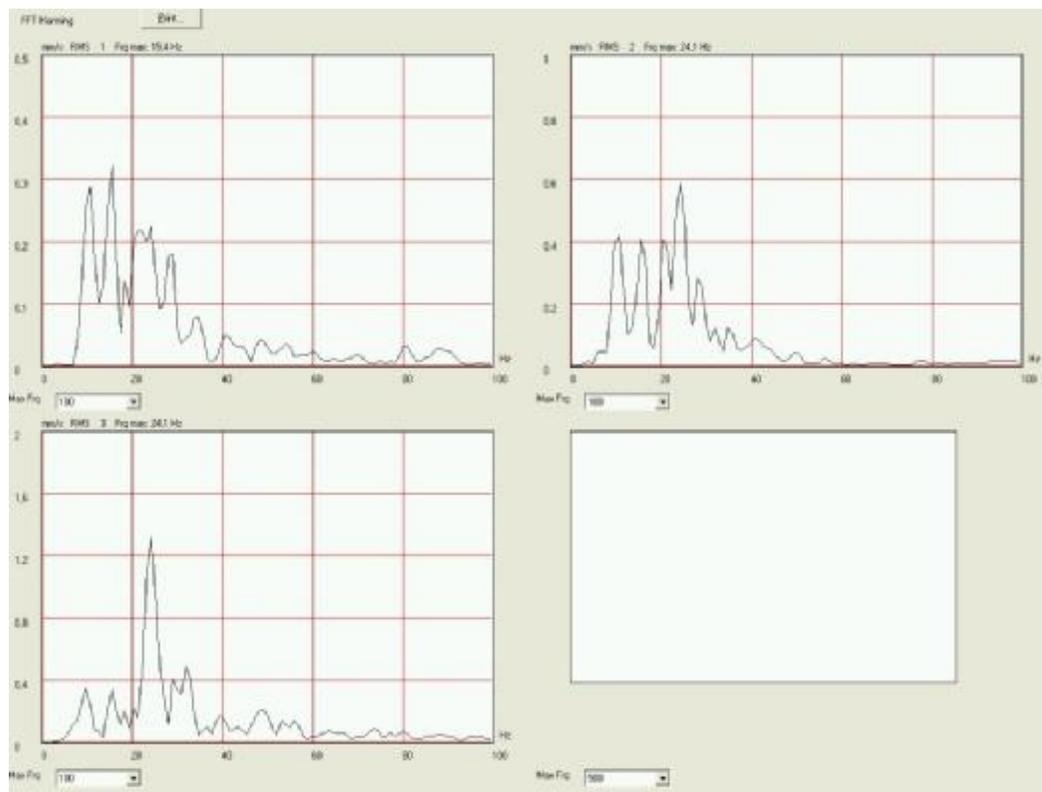
*Fig. 9b The frequency analysis of the vibration of the components (in the longitudinal, transverse and vertical directions) on the measuring position 2 – residential building, on the 3. blast. The measured values are given in Table 3*
