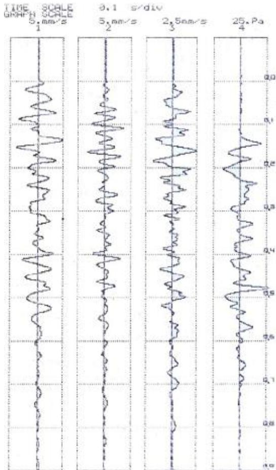
**Fig. 8a** The resulting record the particle vibration and sound waves on the position of one – residential house measured at the 3. blast
