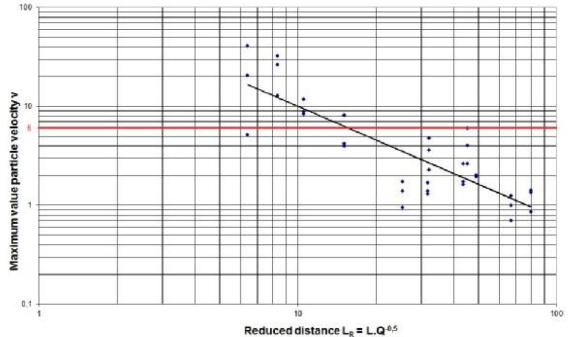
**Fig. 12 Plot of the maximum particle velocity components to reduce the distances at line blasted in the Kučín quarry – law attenuation of seismic waves**
