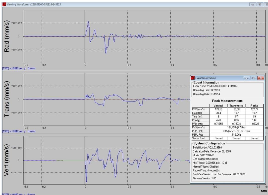
**Fig. 11 Seismic record of particular vibration components vertical-z, transversal-y, longitudinal-x at blast point No. 4049 at the distance of 11.87 m from the first initiated borehole of bench blasting No. 4049 in the quarry Včeláre**
