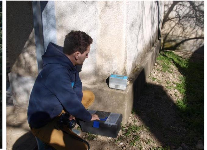
*Fig. 6b The measuring instrument ABEM Vibraloc set on the concrete basis at the entrance of the church*
