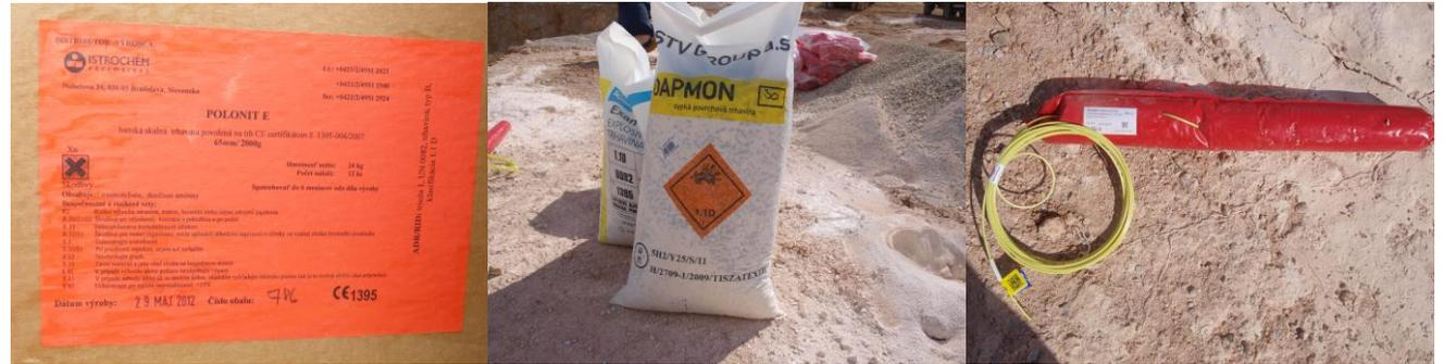
**Fig. 10 Applied explosives in blasting Polonit E, Infernit and Dapmon**
