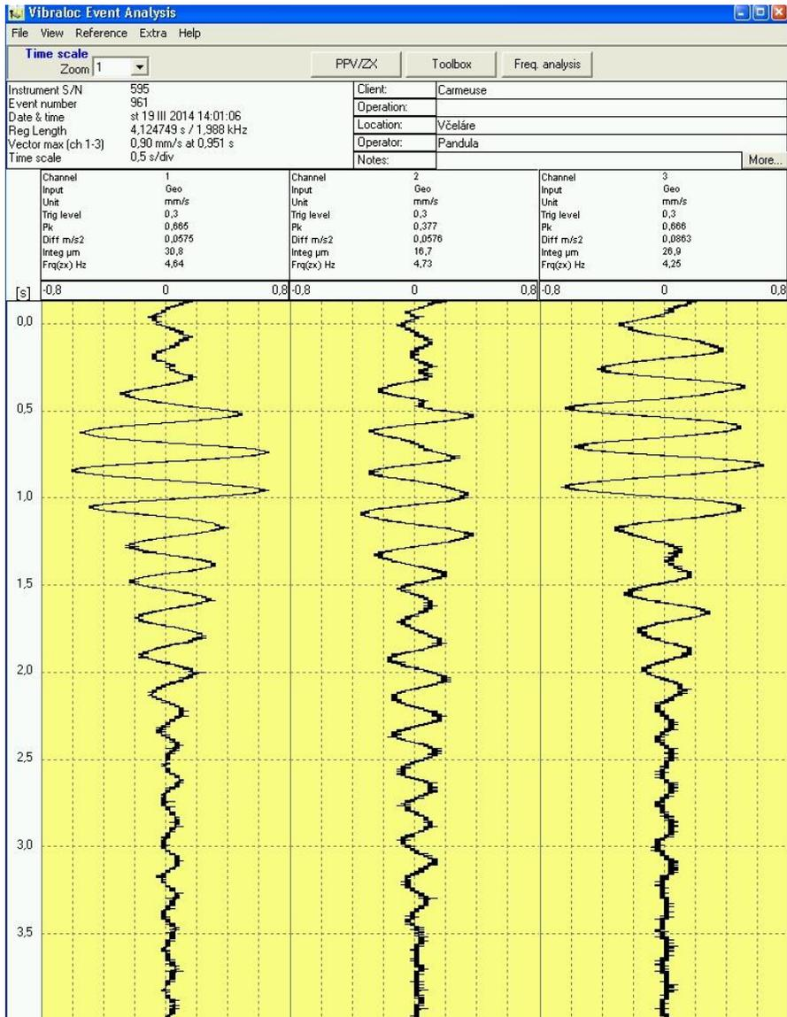
**Fig. 12a** Seismic four-second record of particular vibration components measured at the church in the village Včeláře. The first channel-z, the second channel-x, the third channel-y at the blast point No. 4049
