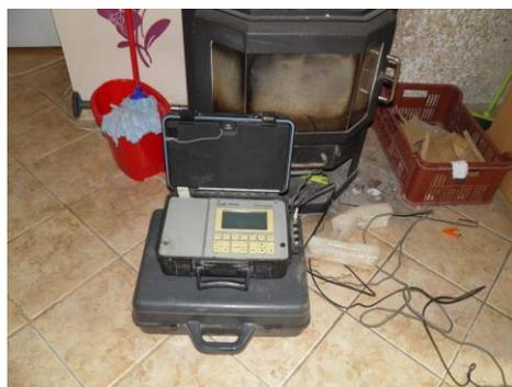
**Fig. 5b** *Position of the seismograph UVS 1504 at the entrance of the family house No. 16 in the village Včeláre*
