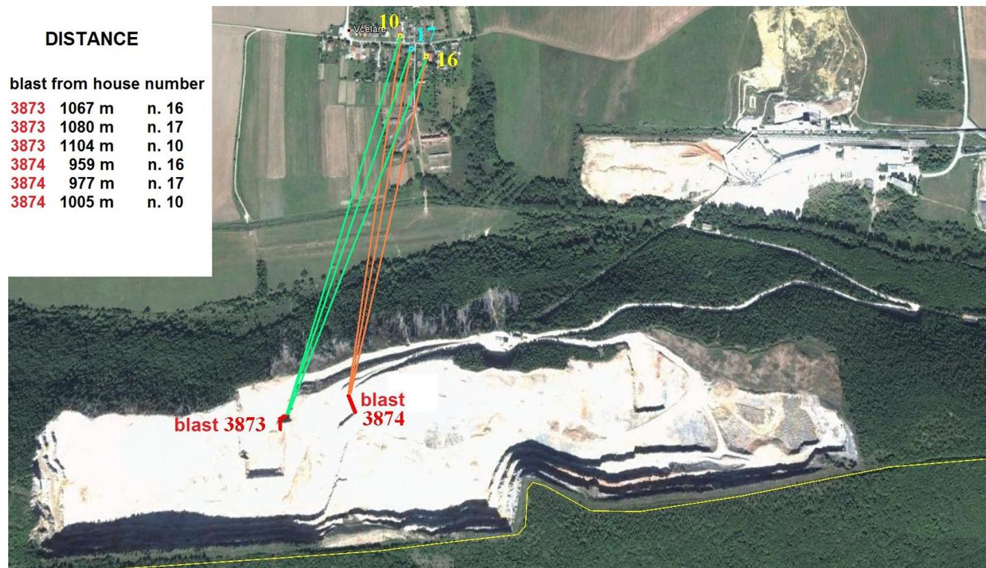
**Fig. 2** Position and distance blast point No. 3873 and blast point No. 3874 in the quarry Včeláre in relation to the measuring standpoints in the village Včeláre
