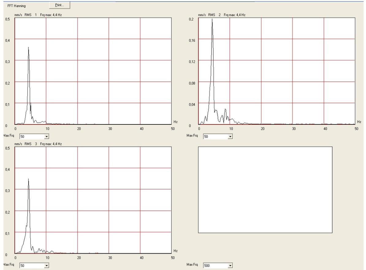
**Fig. 12b** Fourier amplitudes of individual vibration components measured at the church in the village Včeláře. The first channel-z, the second channel-x, the third channel-y at blast point No. 4049
