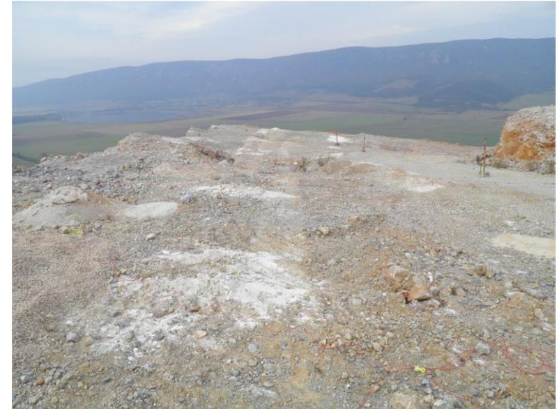
*Fig. 8b Position of boreholes for the bench blasting No. 3874*
