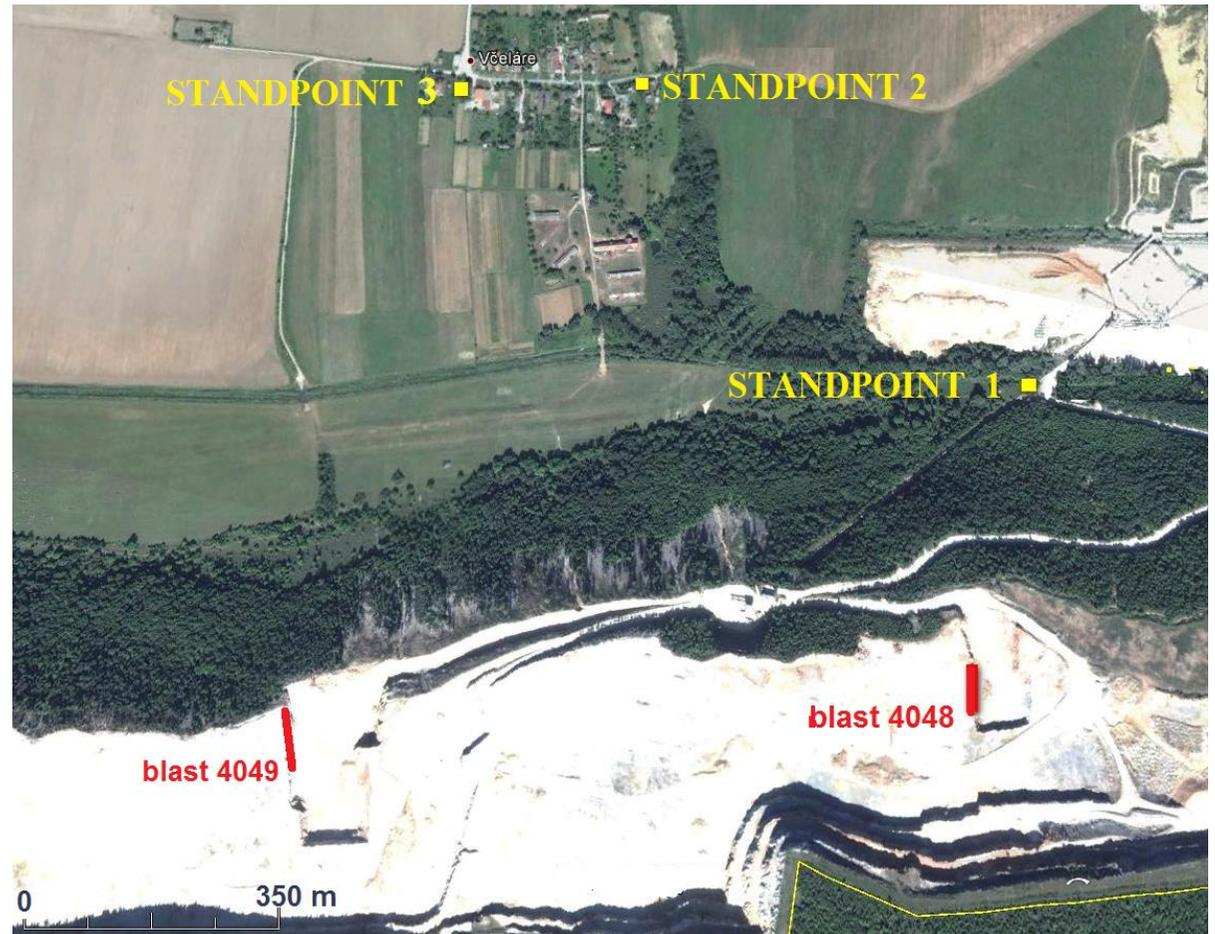
**Fig. 3** Position and distance blast point No. 4048 and blast point No. 4049 in the quarry Včeláře in relation to the measuring standpoints in the village Včeláře
