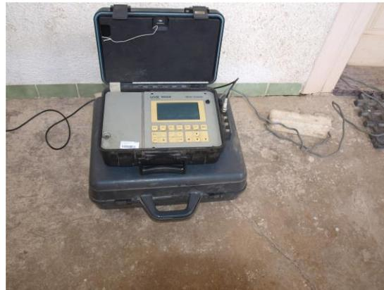
*Fig. 7b The measuring instrument UVS 1504 set on the concrete basis at the entrance of the house*
