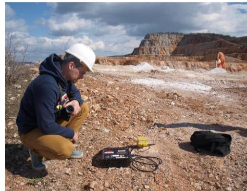
**Fig. 4a** *The position of the measuring standpoint in the quarry Včeláre near to the blast point. The instrument VMS 2000 MP in distance of 11.87 m from the boreholes of the bench blasting No. 4049*
