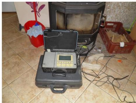
**Fig. 5b** *Position of the seismograph UVS 1504 at the entrance of the family house No. 16 in the village Včeláre*
